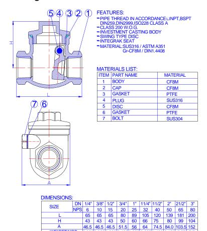
The name of the various component of Swing Check valve(B)
